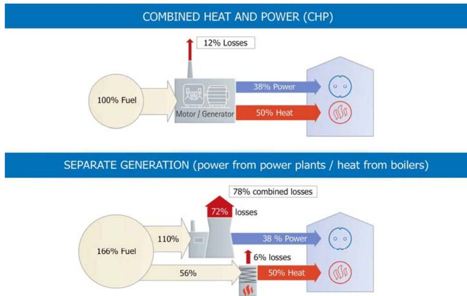
Figure 2: the primary energy benefit of cogeneration (@ Bundesverband Kraft-Wärme-Kopplung)
