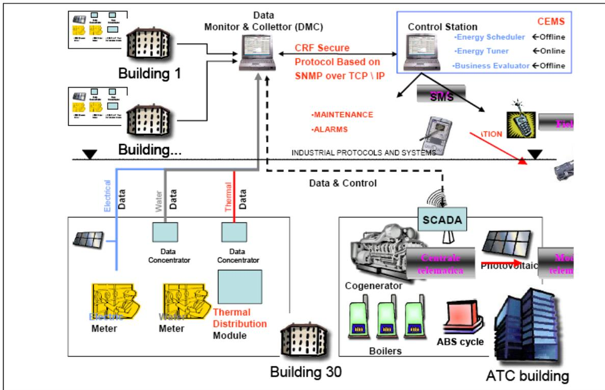
Figure 2. I-CEMS Functional Architecture
