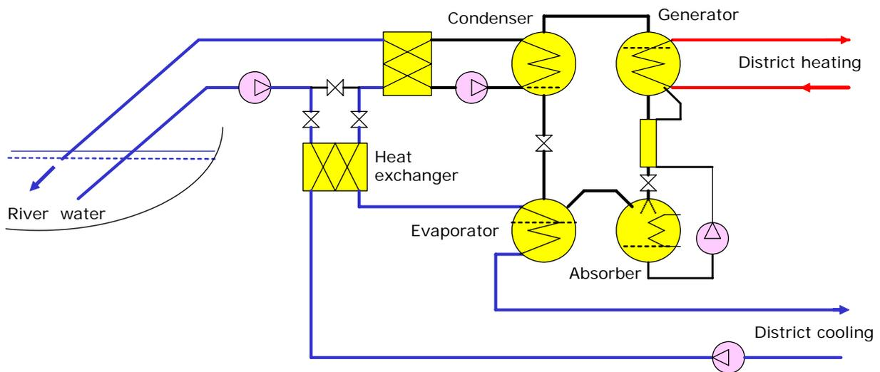
Figure 2. Principle of cold production plant with heat exchangers and absorption chiller.
