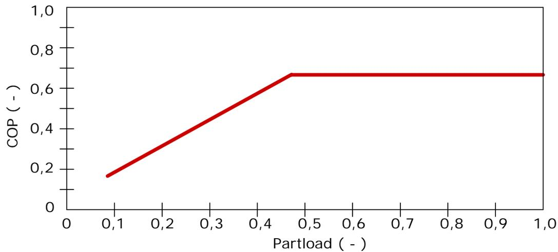
Figure 7. Coefficient of performance (COP) at part load operation
