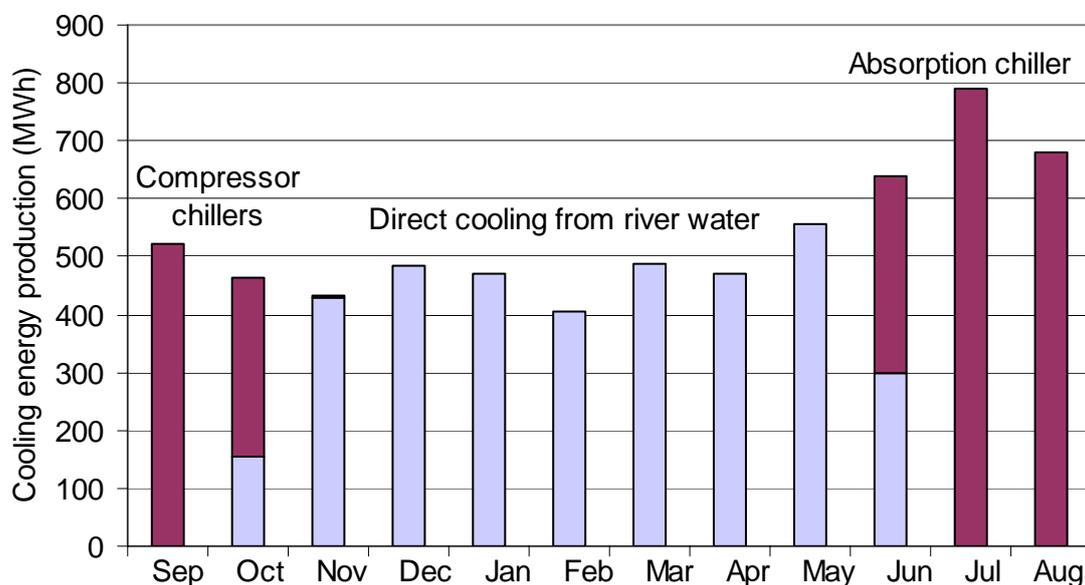
Figure 6. Cold production from different cooling sources from September 1. 2006 to September 1. 2007
