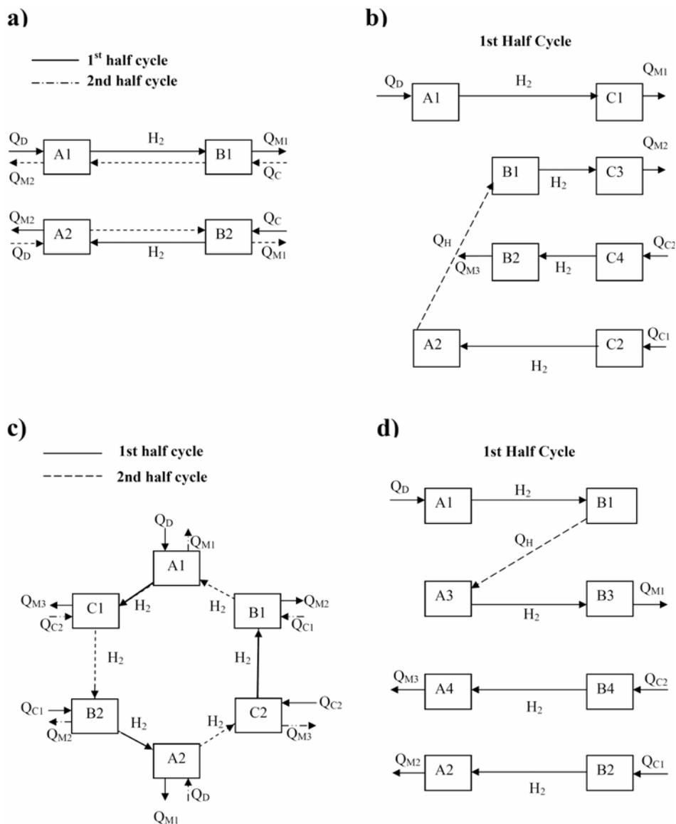
Figure 2. Different Sorption Cooling System Configurations
