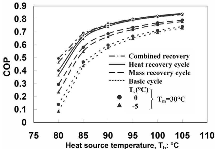
Figure 4: Effect of Heat & Mass Recovery on Cooling System Performance [28-30]
