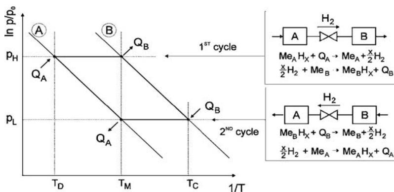
Figure 1: Operating principle of a single stage metal hydride heat pump
