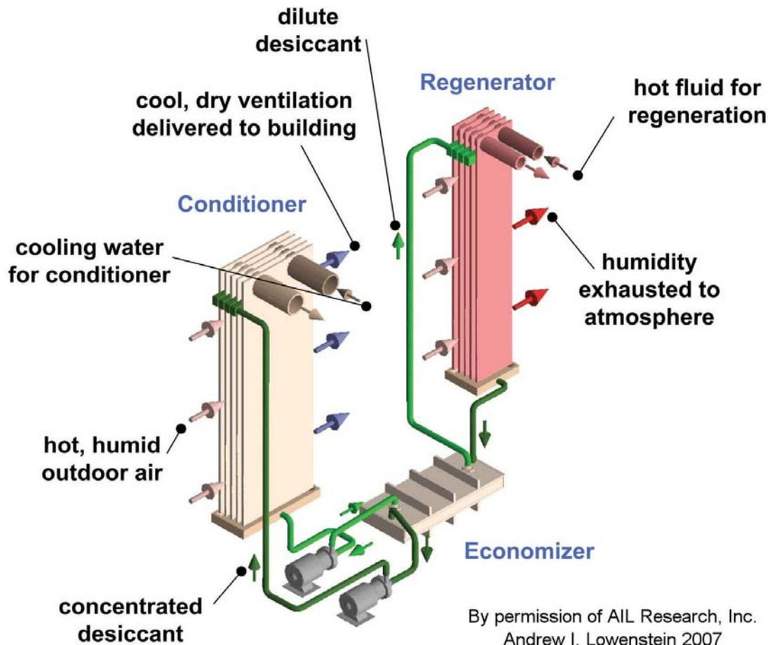
Figure 9. 3-D schematic of an AIL Research Liquid Desiccant dehumidifier.
