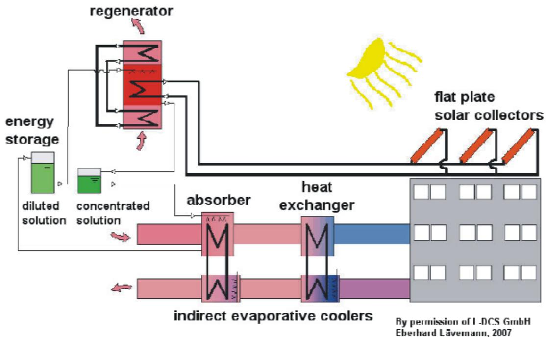
Figure. 8 -Schematic representation of a solar-driven L-DCS plant.
