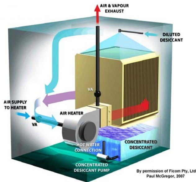
Figure 7. Schematic 3-D view of Ficom's desiccant regenerator.
