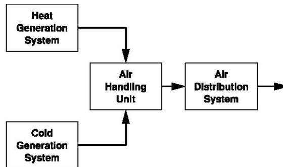
Figure 3 -Block-diagram of a conventional central airconditioning system.
