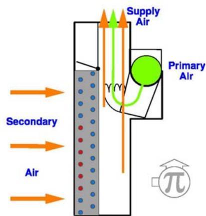
Fig. 13 - Schematic illustration of an induction unit.
