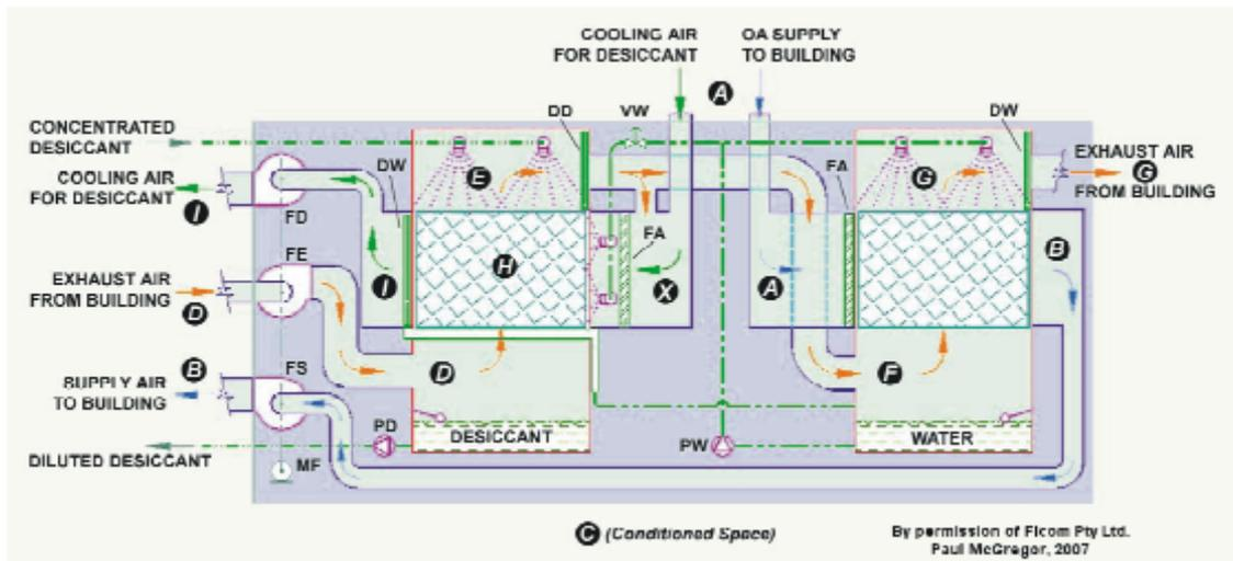
Fig. 6 -Schematic representation of Ficom's AHU.
