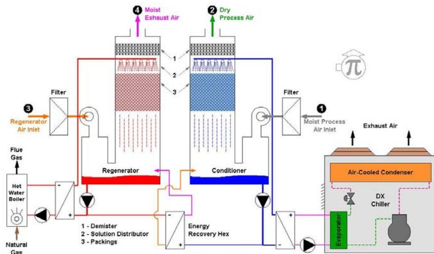
Figure 4 -Author's representation of a typical Kathabar system.
