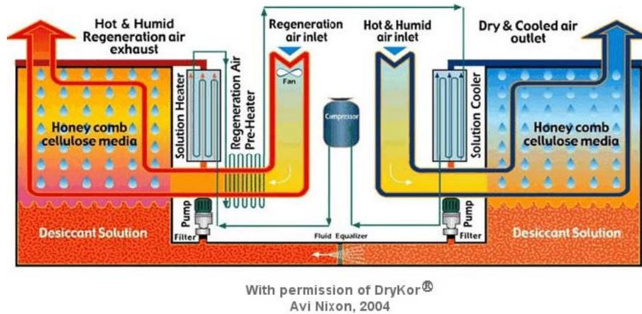
Fig. 5 -Schematic representation of a DryKor® air dehumidifier.
