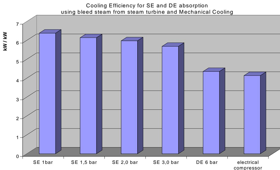
Figure 1. Cooling efficiency of different systems
