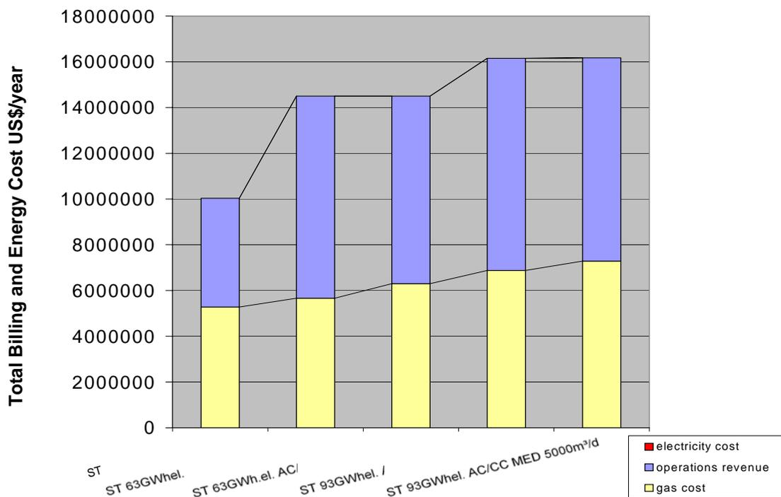
The five columns show the total income and the gas cost for the boiler for different modes of operation
