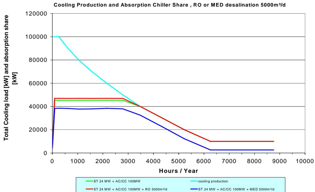
Figure 2: share of absorption chiller load for MED and RO system scenarios , for reference no desalination - green line
