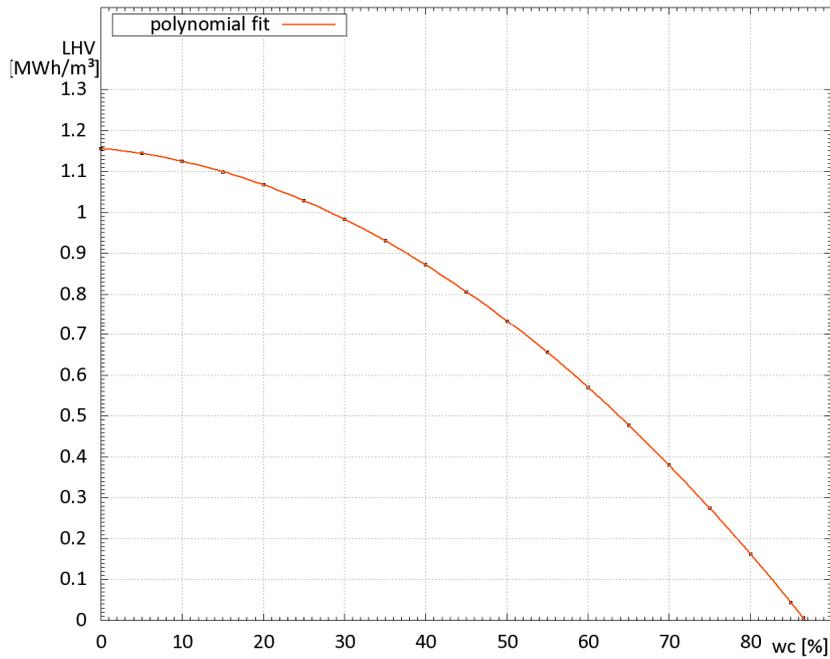
**Figure 3: Net calorific value (NCV/LHV) as a function of fuel water content.**
