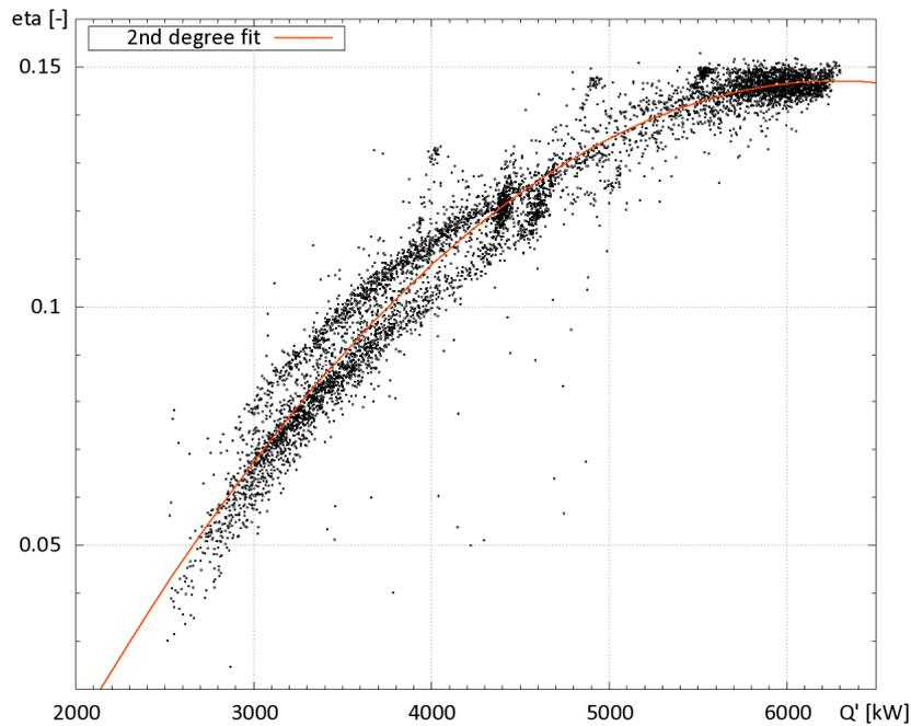
**Figure 4: electric gross efficiency vs. thermal input (2008)**
