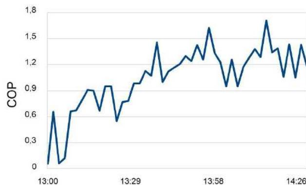
**Figure 4: Instantaneous COP of the absorption GCHP**
