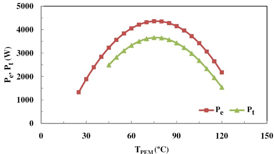
Figure 4. Thermodynamic efficiency, electric and thermal power as a function of temperature
