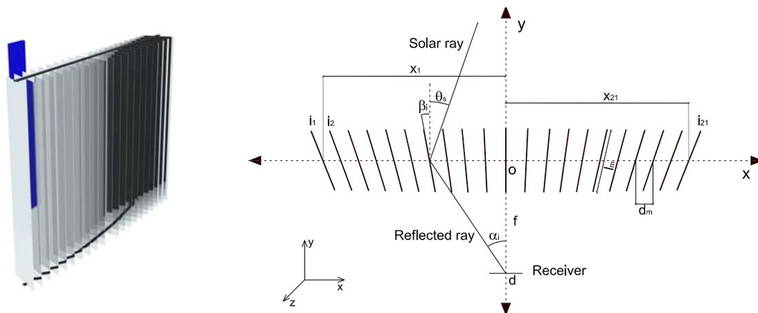
**Figure 1: On the left: Fresnel reflector 3D view and on the right: Fresnel concentrator schematic.**
