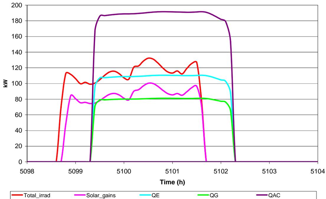
**Figure 4: Evolution of the Energy performance of the CS solar cooling system on 1<sup>st</sup> August of a Typical Meteorological Year**
