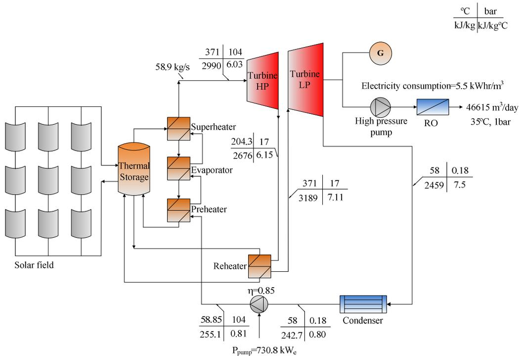
Fig 7: Simulation of RO facility integration into a PT-CSP plant
