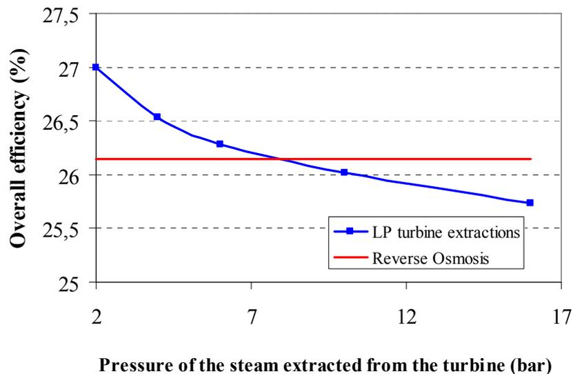
**Fig 8: Comparison of the overall efficiency obtained with different LT-MED-TVC configurations (steam extraction at different pressures) against RO unit**
