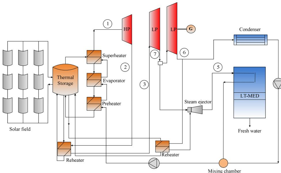
**Fig 3. Diagram of the LT-MED-TVC unit integration into a PT-CSP plant, considering extraction from the LP turbine**
