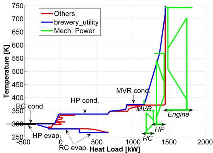
Figure 6: CHP System+MVR, Heat Pump Condensing at 66.5°C, COP=5.37 (solution 4)
