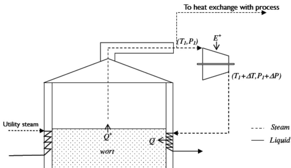
Figure 5: Mechanical vapor on the wort evaporation
