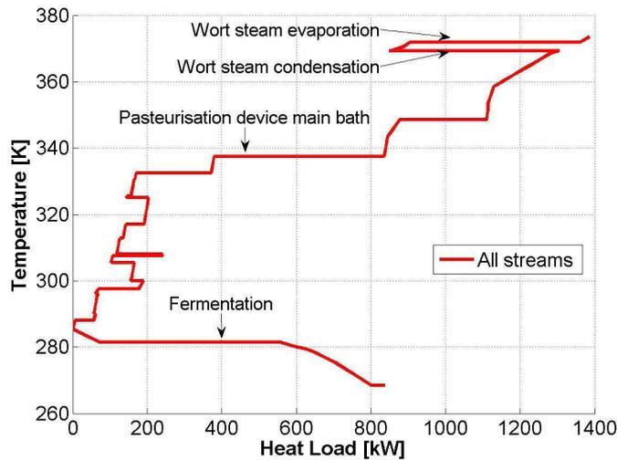
Figure 2: Grand composite curve of the process
