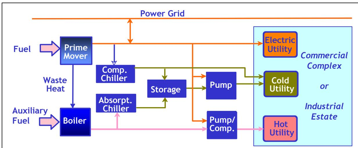
**Figure 1: Schematic presentation of cogeneration and district energy (CDE) network**
