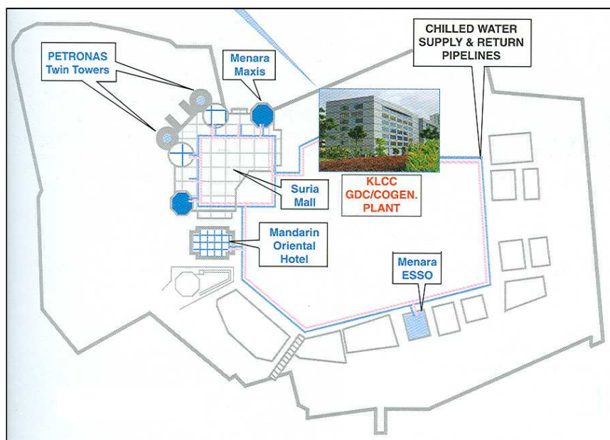
Figure 3: Cogeneration and district cooling network in KLCC
