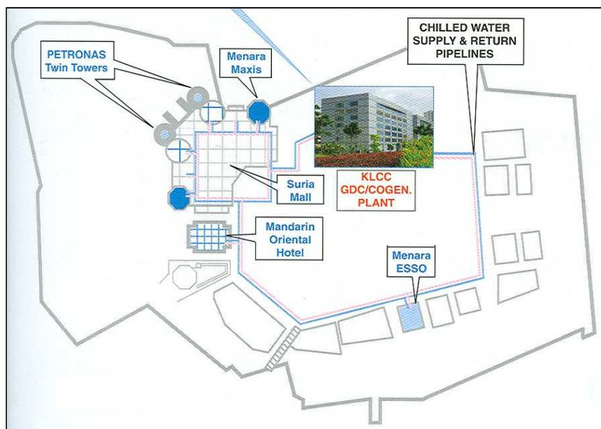
**Figure 3: Cogeneration and district cooling network in KLCC**
