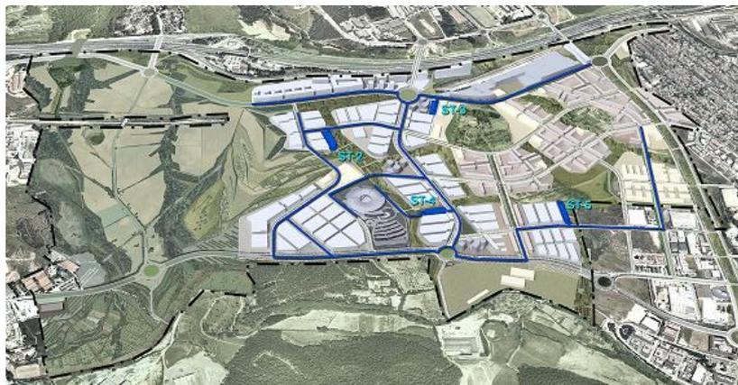
Figure 2. District Heating and Cooling network and location of the cogeneration plants.
