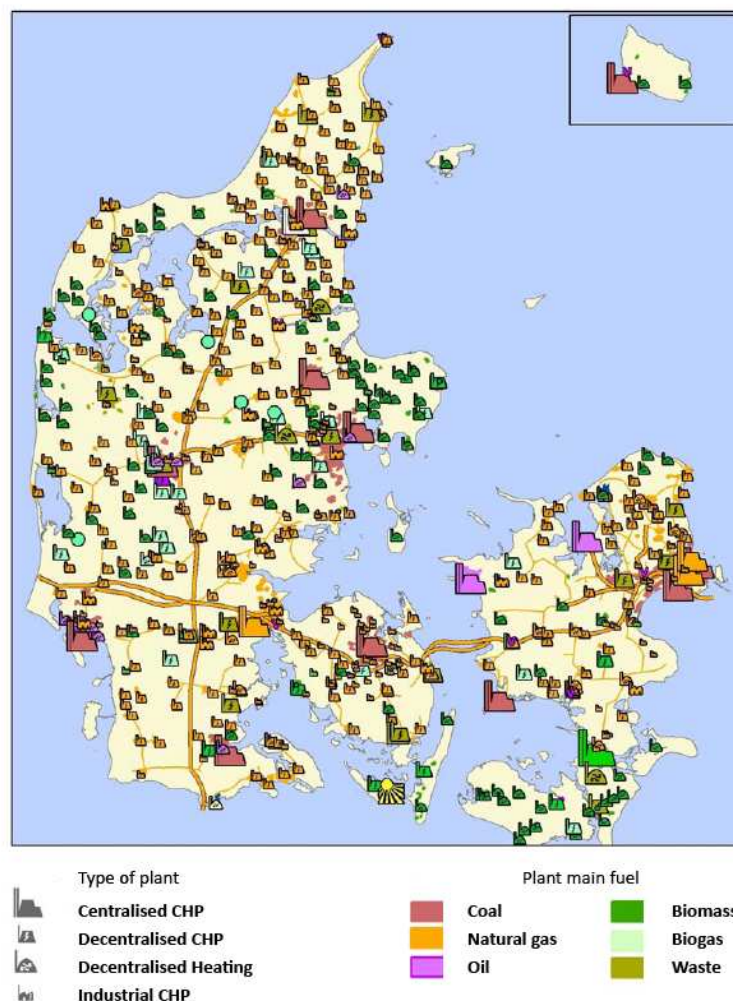
Figure 1: Denmark Energy Map 2004 – CHP and heating stations [2]
