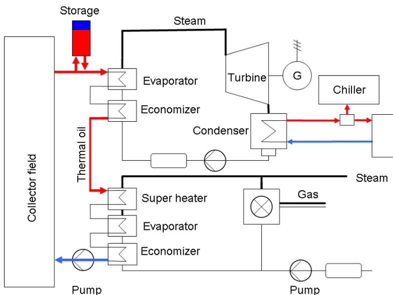
**Figure 1: Possible cycle layout for solar polygeneration.**
