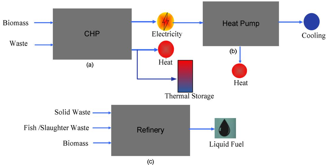
**Figure 3: Quadgeneration energy system with existing district heating plant. Case studies and Results Discussion**
