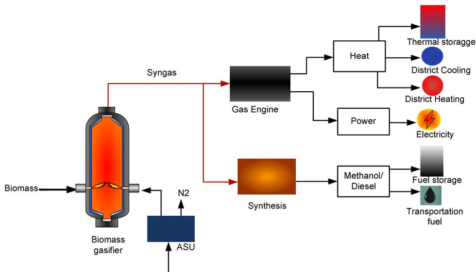
**Figure 4: Quadgeneration energy system with gasification unit.**
