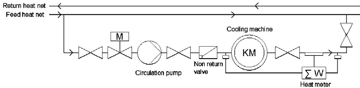
**Fig. 3: Direct connection of the cooling machine to the district heat net**
