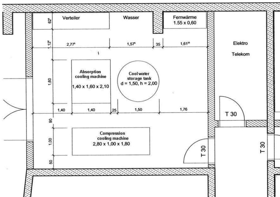
Fig. 2: Floor plan of the central heating room in the Elektror building
